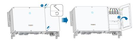
**step 3** Keep the wiring compartment open during wiring through the limit lever attached to the cover.
