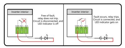
figure 5-8 Normal open contact
