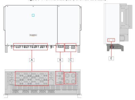
figure 5-2 Terminal Description(For four single-core cables)
