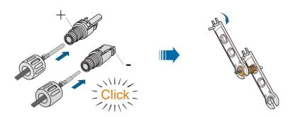
step 4 Check for polarity correctness.
