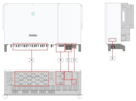
figure 5-1 Terminal Description(For a multi-core cable)
