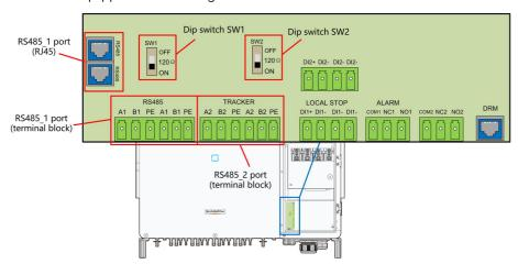
The inverter is equipped with two groups of RS485 communication port for external communication connection, which are RS485\_1 port and RS485\_2 port.
