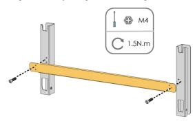
**step 2** Level the assembled mounting-bracket by using the level, and mark the positions for drilling holes on the installation site.
