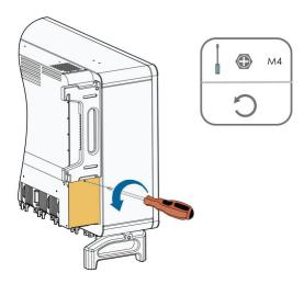
**step 3** Press the tab of the latch hook, unplug the cable connection joint outwards, and loosen the screw on the fan holder.
