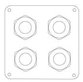
figure 5-3 Spare AC Sealing Plate
