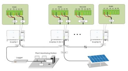
figure 5-5 Multi-inverter Communication System [RS485\_1 Interface (Terminal Block)]
