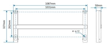
figure 4-1 Dimensions of mounting-bracket
