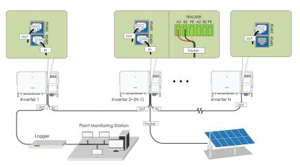
figure 5-6 Multi-inverter Communication System [RS485\_1 Interface (RJ45)]
