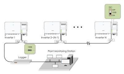
figure 5-7 Configuration of Dip Switch (N≥15)
