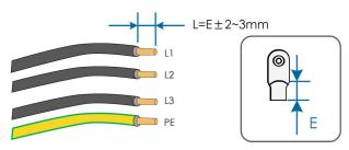
step 6 Make the cable and crimp OT/DT terminal.
