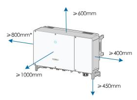
\* In case the distance is less than 800 mm, move the inverter from the mounting-bracket or wall before maintaining fans.
