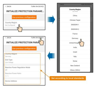
figure 7-4 Initialization Protection Parameter
