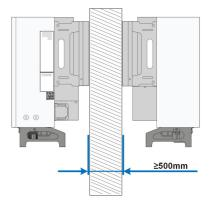
Install the inverter at an appropriate height for ease of viewing LED indicator and operating switch(es).
