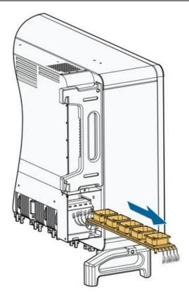
**step 5** Reinstall the fan back to the inverter in reverse order and restart the inverter.
