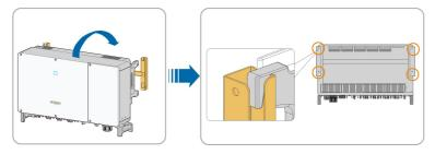
step 4 Fix the inverter with screws.
