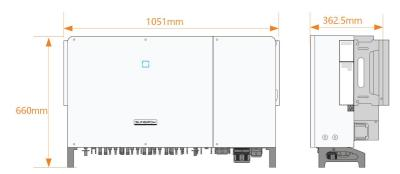
figure 2-3 Dimensions of the Inverter(in mm)
