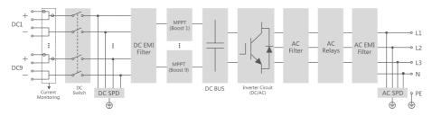
figure 2-4 Circuit Diagram
