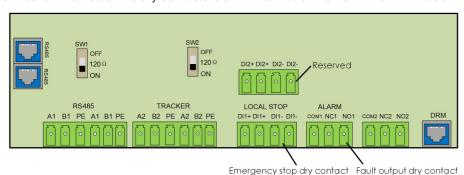
**DO terminal (fault output dry contact):** The relay can be set to output fault alarms, and user can configure it to be a normally open contact (COM & NO) or a normally closed contact (COM & NC).
